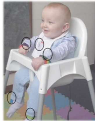
Image: Placement of 5 sensors on an infant's torso, wrists and ankles. Black ovals mark the location of sensors hidden in clothing.
